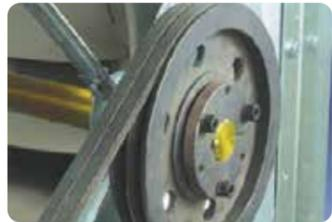
1 Taper Lock Bushing Pulley
